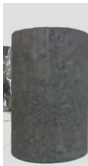
Figure 9. Boric acid treated anode sample after air reactivity test, ARR: 87 %.
